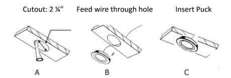
DO NOT PRESS ON LENS TO INSERT PUCK – IT CAN DAMAGE PUCK
